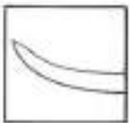
SS-21-362 Curved 3 mm curve from tip
